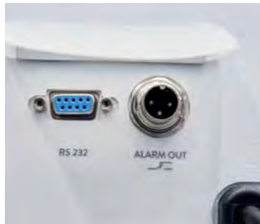
Standard-issue RS 232 interface and alarm contact
